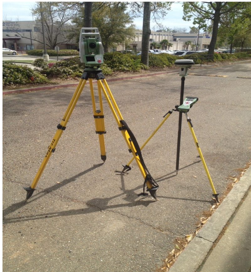
Figure 1: Photograph of Leica TS15 Total Station and Leica CS/GS15 GPS uni
