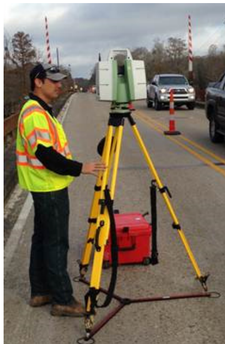
Figure 2: Photograph of Leica ScanStation C10
